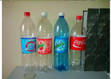
3f. The used soft drinks bottles can be used to measure volume of 1.5 litre. For timing, you can easily use your watch. You will need to record the time taken to fill up a bottle. The timing is the data that you require.
